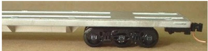
This car is fitted with trucks in the scale position, and with body mounted couplers
