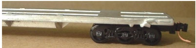
For comparison, this car is fitted with truck mounted couplers (trucks nearer end of car)
