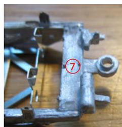
⑦ The brake cylinder and 3 way valves are placed on the articulated ends of the A, B and D cars only, taking care to allow room for the walkway.
